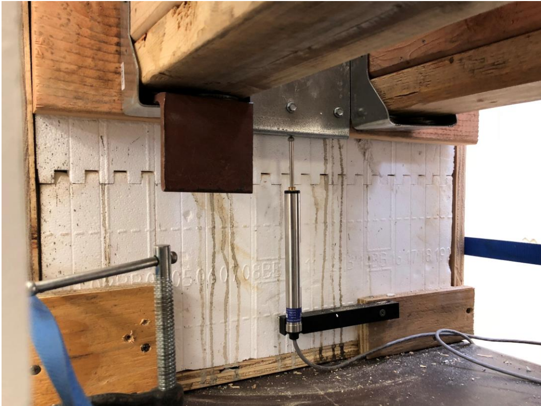
Figure 3. Test Setup- Right Joist Hanger
