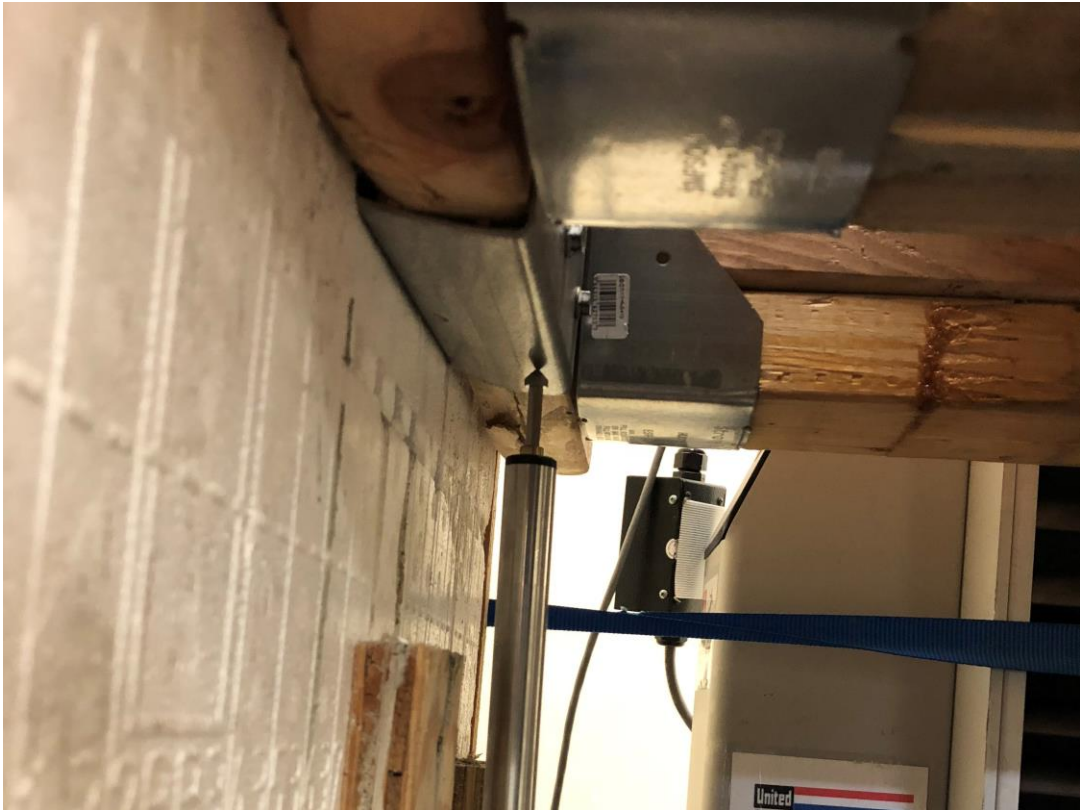
Figure 1. Typical failure mode of specimen at ultimate load
